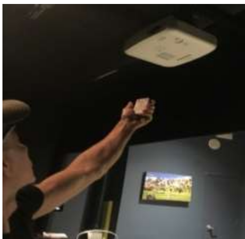
From the front of projector, aim the the remote at the lens and press RED Button 2 times. Green light indicates it's ON
