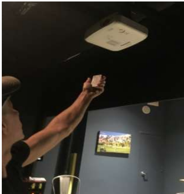
From the front of projector, aim remote projector lens and press red button. Green light indicates it's warming up.
